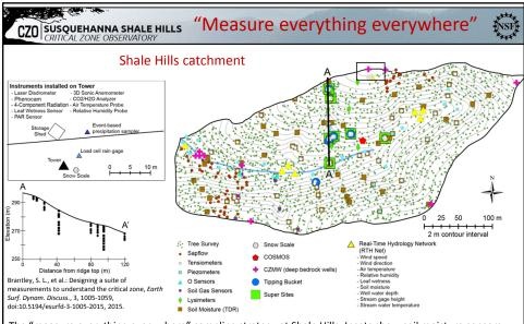
The "measure everything everywhere" sampling strategy at Shale Hills. Insets show soil moisture sensors (circles) and lysimeters (squares) along the transect shown on the map. Sensor and lysimeter depths are exaggerated five times compared to the land surface elevation. Second inset shows instrumentation deployed at the meteorological station on the northern ridge. Small green dots are the surveyed and numbered trees.
