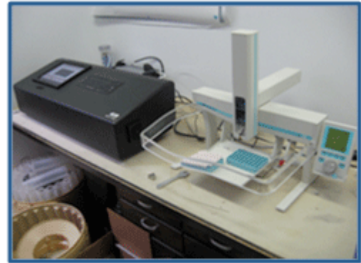
Figure 3. DLT-100 liquid water stable isotope analyzer, with auto-injection unit, from Los Gatos Research.
