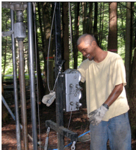
Figure 2a) Terryl Daniels (PSU undergrad) drills wells with the Portadrill Mini.
