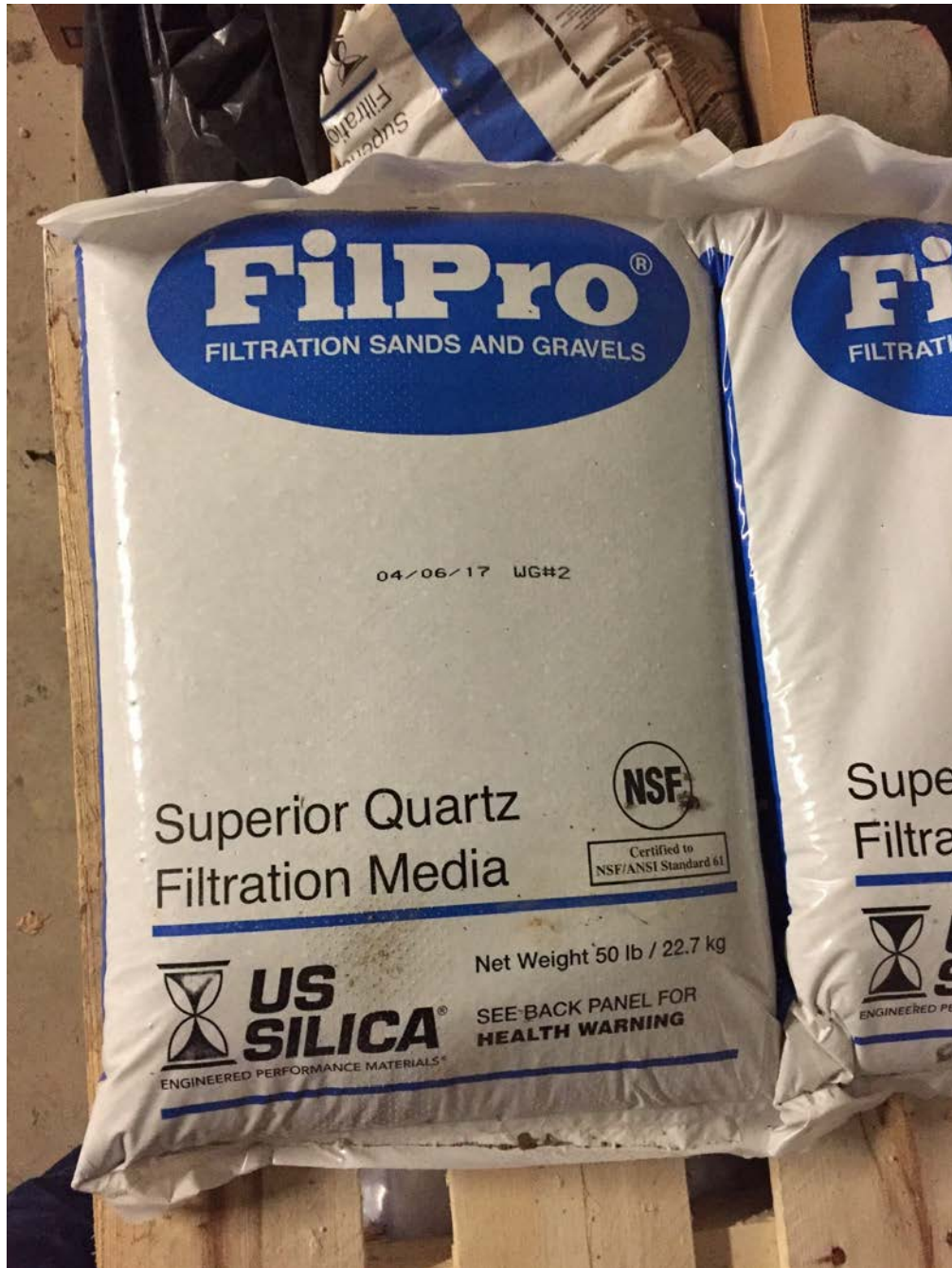
FilPro Quartz Filtration Sand (#2 size) used as the filter pack in monitoring well CZMW-4
